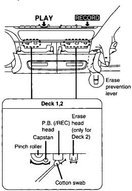
It is recommended that the head assembly be demagnetized if distortion or poor sound quality persists after cleaning the heads.
